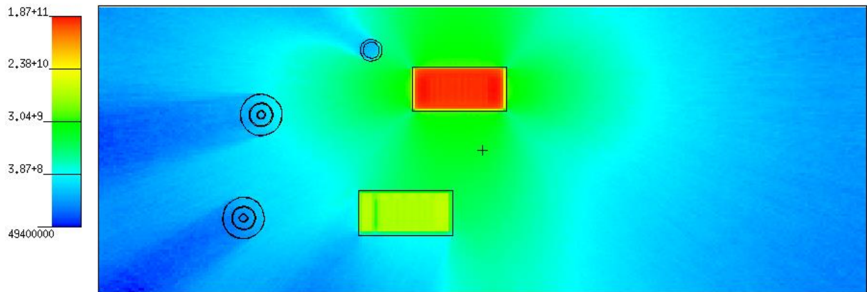
Figure 15. Gamma flux profile at time 6419 (gammas/cm 2 -s). At this time, fuel baskets had been removed from the OR, and the ER was processing fuel.
